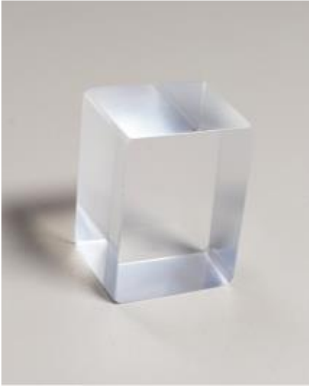
Figure 1. Experimental block (EMB) made only of resin matrix. The size of the block is 18 \times 15 \times 15 mm.
