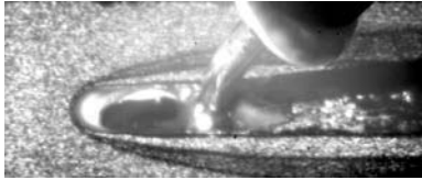
Fig.1 High-speed image during welding (optimum welding).
