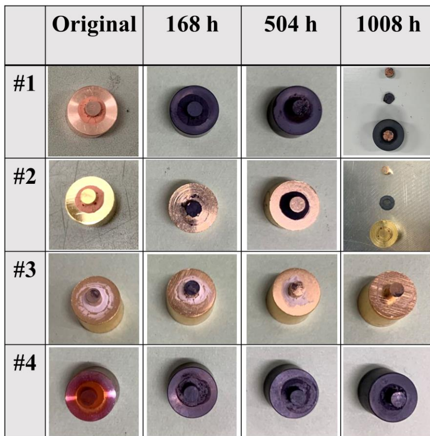
Figure 5.1 Joint samples prepared with different conditions after ageing for various time intervals.
