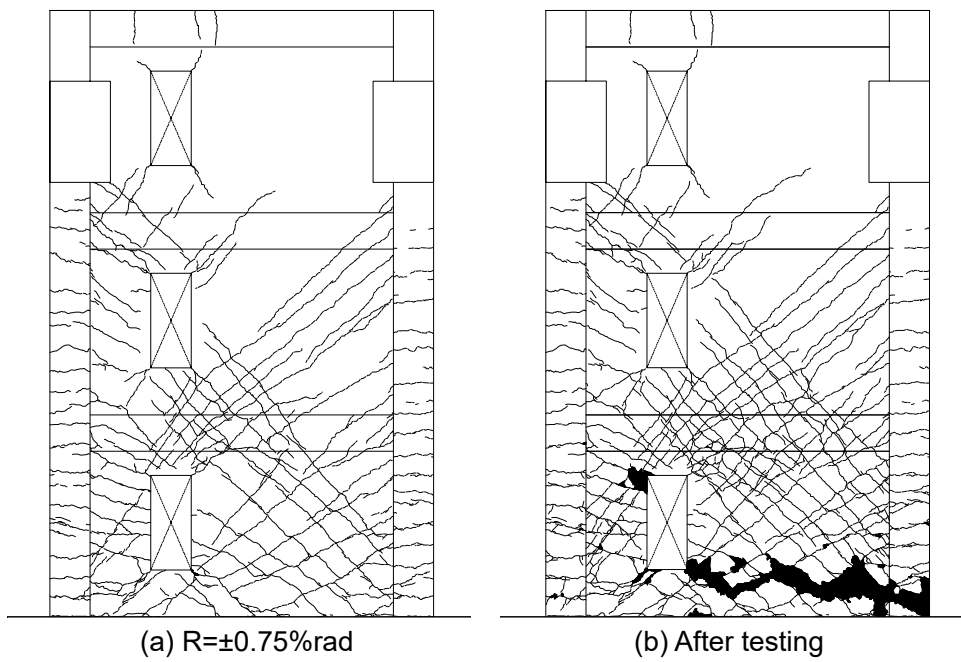
Fig.6.3.2 Damage to WW6
