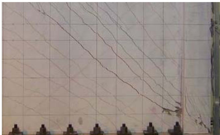
(a) Failure of the wall bottom ( R=+1.0\% rad)
