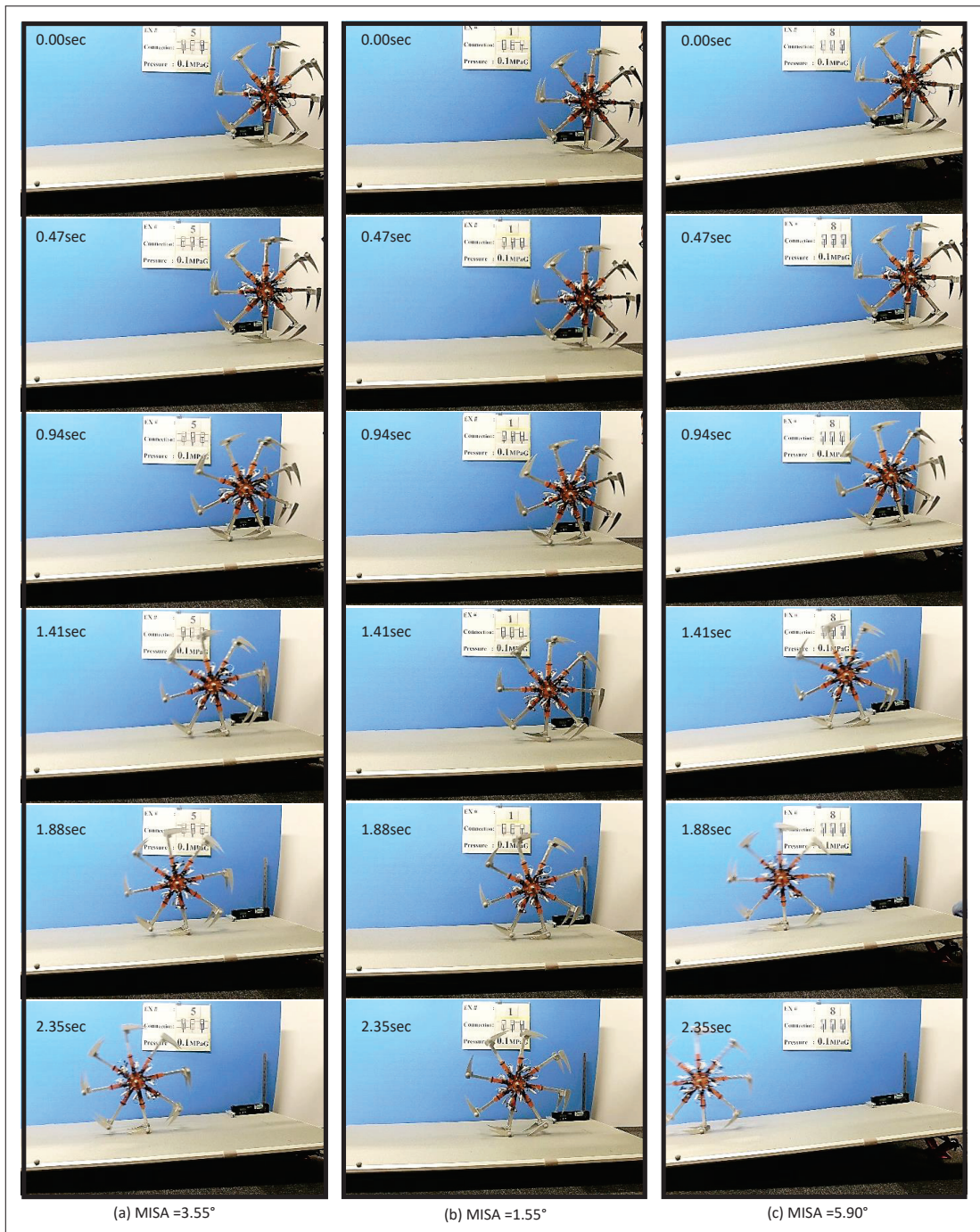
Figure 3.12: Time-series photographs of OCTANS with 0.10 MPaG pressurized ANS during locomotion, showing one of the commonly occurring MISAs across 10 trials under (a) condition 1, (b) condition 2, and (c) condition 3, after increasing the slope angle gradually until the robot started moving. The interval between two pictures is 0.47 s.
