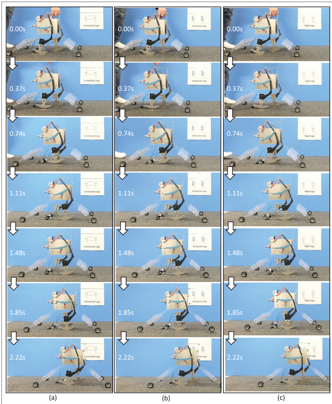
Figure 4.8: Time-series photographs of one gait cycle of the bipedal robot during locomotion, showing one of the conducted trials of each connection pattern. (a) Type 1, (b) Type 2, and (c) Type 3. The interval between every two successive pictures is 0.37 s.
