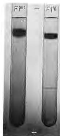
FIGURE 3. Polyacrylamide disc gel electrophoresis of Fi^{mt} and Fi^{fg} . The gels contained 7% acrylamide, 0.2% N, N' -methylene-bis-acrylamide, deionized 8 M urea and 0.375 M Tris-HCl buffer, pH 8.6. Electrophoresis was run at a constant current of 3 ma per tube for 150 min at +C.
