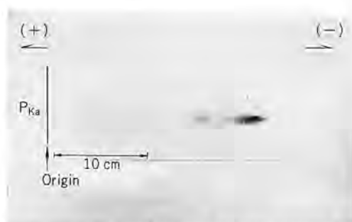
FIGURE 9. High-voltage paper electrophoresis of P_K in pyridine-acetate buffer, pH 6.5. 200 \mu g of P_{Ka} were applied. Electrophoresis was carried out by applying 50 v/cm for one hr and 35 v/cm for another hr. The peptides were located by the ninhydrin reaction (showed in this figure) and later with peptide stain.
