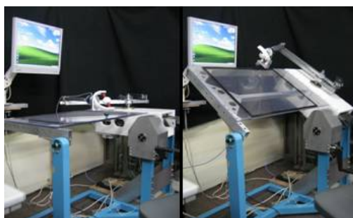
図 4-38 Quasi-3-DOF Rehabilitation System “PLEMO”
