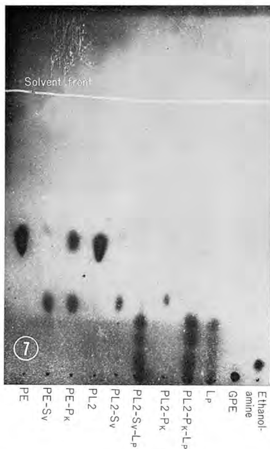
FIGURE 7 TLC of PE, PL2 and their breakdown products. (Ninhydrin, Solvent I)
