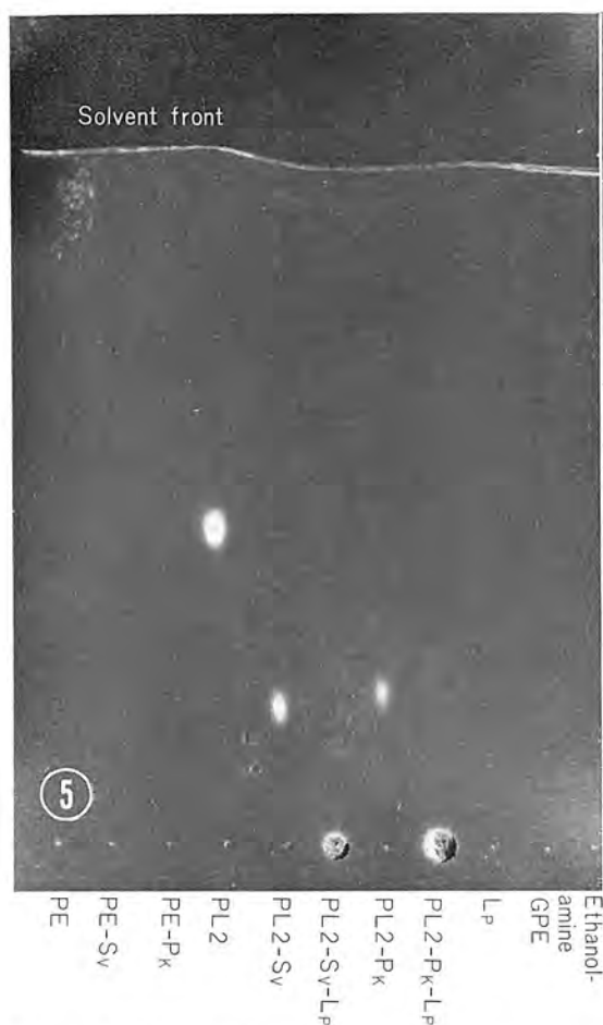
FIGURE 5 TLC of PE, PL2 and their breakdown products. (Autoradiography, Solvent I)
