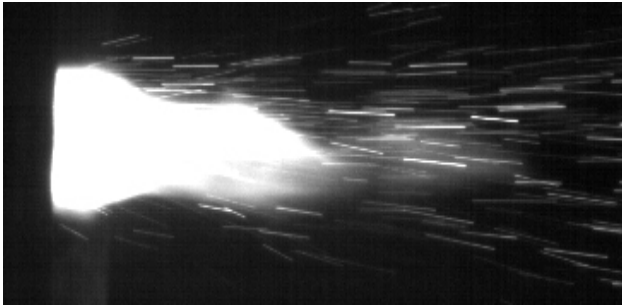
Fig.9 A picture of plasma plume with \text{Al}_2\text{O}_3 powder
