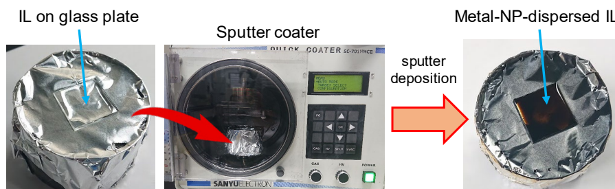
Figure 1. Schematic diagram of procedure for ionic liquid-sputtering method.
