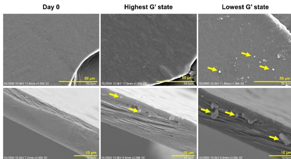
Figure 2-10. Surface and cross-section morphology of dried TCNF/NTS film prepared with suspension at day 0, the day yielding the highest G' and the day yielding the lowest G' . Starch granule on film surface and cross-section indicated by yellow arrow.
