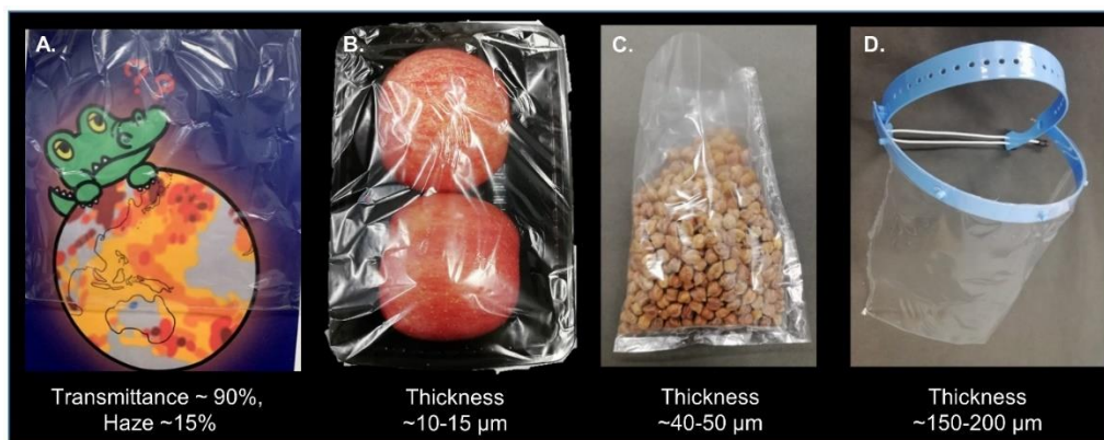
Figure 2-12. (A) TCNF/HPS films exhibit high optical transparency. The film thickness can be optimized according to its use in (B) food packaging covers ( \sim 10\text{-}15 \mu\text{m} ), (C) packaging bags ( \sim 40\text{-}50 \mu\text{m} ), or (D) face shields ( \sim 150\text{-}200 \mu\text{m} ).
