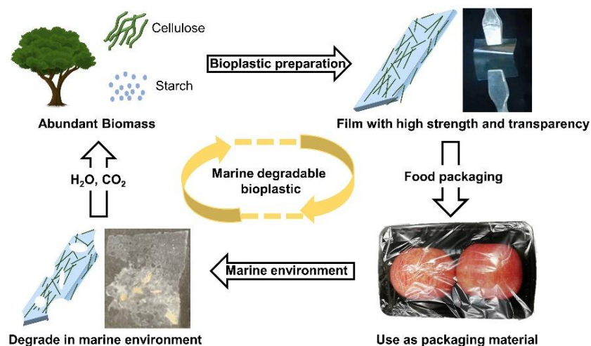
Fig. 1. Concept of polysaccharide based packaging film to reduce marine pollution.
