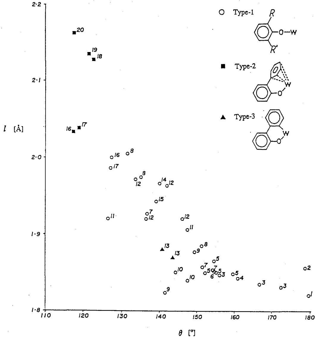
Fig. 3-6. Coordination geometry of phenoxy ligand in the molecular structures of tungsten-phenoxydes by the W-O bond distance [ $l$ ] vs. W-O-C bond angle [ $\theta$ ] plotting.<sup>25)</sup>
