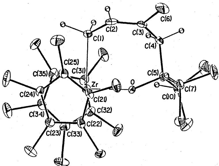
Fig. 2-7. Molecular structure of **7** projected onto the plane defined by Zr, O, and C(1) atoms.
