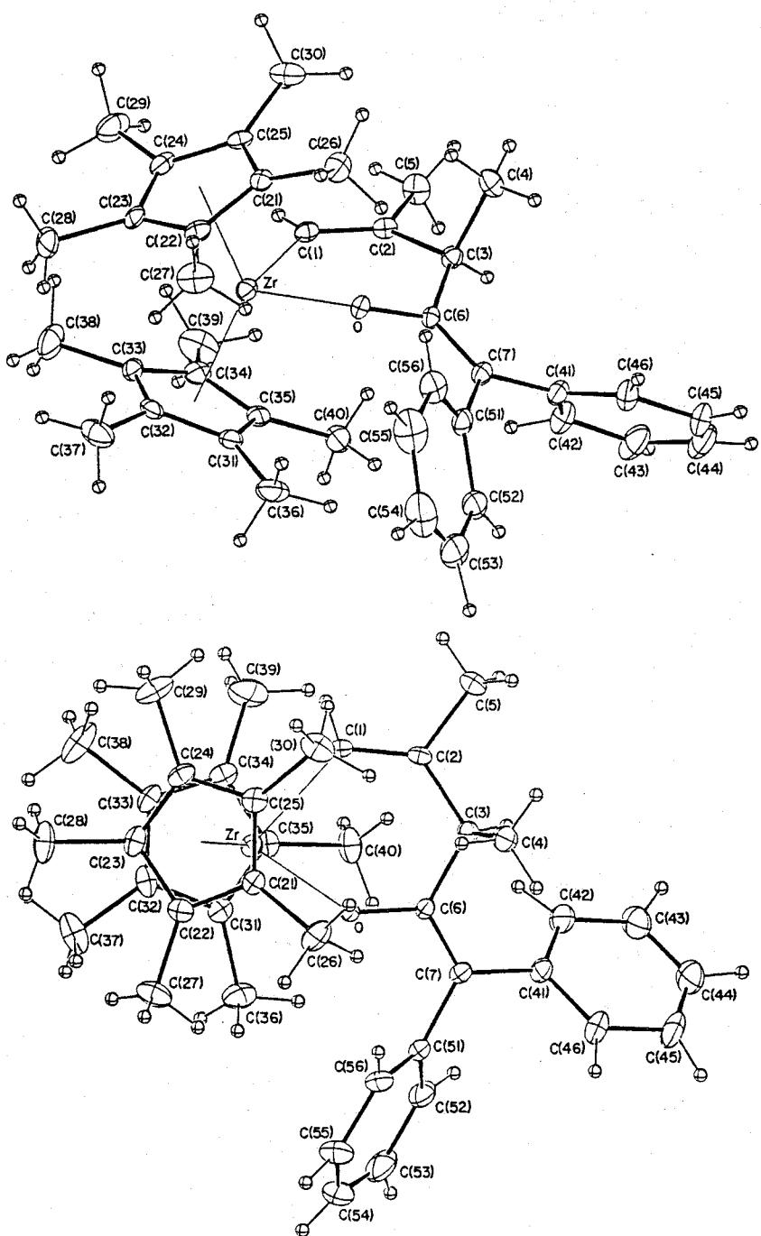
Fig. 2-4. Molecular structure of  $(\eta^5\text{-C}_5\text{Me}_5)_2\text{Zr}(\text{isoprene})((\text{C}_6\text{H}_5)_2\text{C}=\text{C=O})$  (5).
