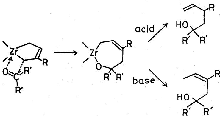
Hydrolysis of 7 with protic acid (aq HCl) gave 2,5-dimethyl-3-isopropyl-6-hepten-3-ol but hydrolysis with bases such as NaOH and Et<sub>2</sub>NH gave (Z)-2,5-dimethyl-3-isopropyl-5-hepten-3-ol quantatively, in line with the X-ray structure. The high regioselectivity observed in the formation of 7 is explained by the inductive effect of the methyl group of isoprene, which causes the higher negative charge on the C<sub>1</sub> atom.
