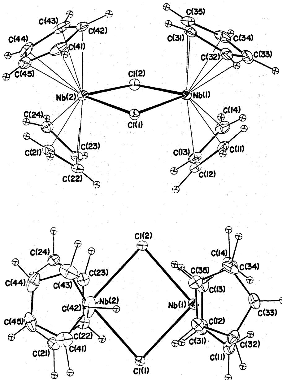
Fig. 1-9. Molecular structure of  $[(\eta^5\text{-C}_5\text{H}_5)\text{Nb}(\mu\text{-Cl})(\text{C}_4\text{H}_6)]_2$  (34).
