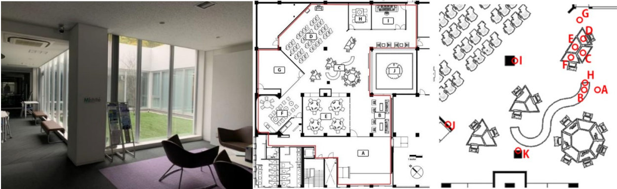
Figure 11: (left) the lounge area in the selected case study. (middle) different functional areas within the selected case study, the measurement points included in the study are in areas C and D, J represents the courtyard. (Right) Sensor points selected for comparison, points H, I, J, and K are on vertical surfaces.
