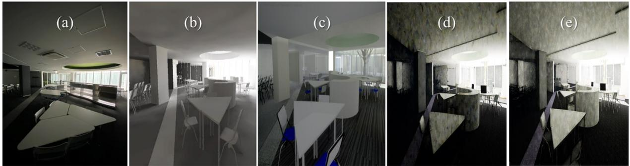
Figure 12: A point-in-time view at 11:00 am for the test environment, and its corresponding simulation outputs in different techniques. (a) real space, (b) Radiance, (c) UE4 with no RTX, (d) UE4 RTX 3 bounces, (e) UE4 RTX 7 bounces.
