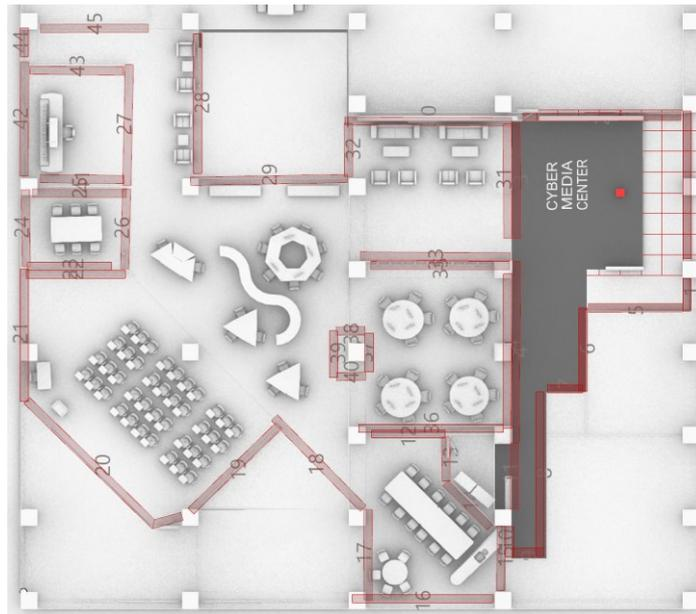
Figure 29: Generated mesh volumes for walls marked by unique index numbers, both sides of each interior wall were generated separately.
