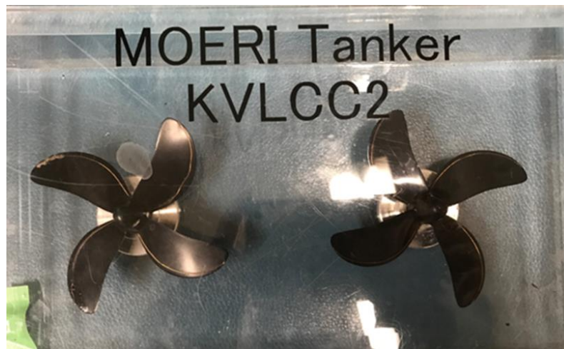
Figure 2-6 MOERI Propeller models.
