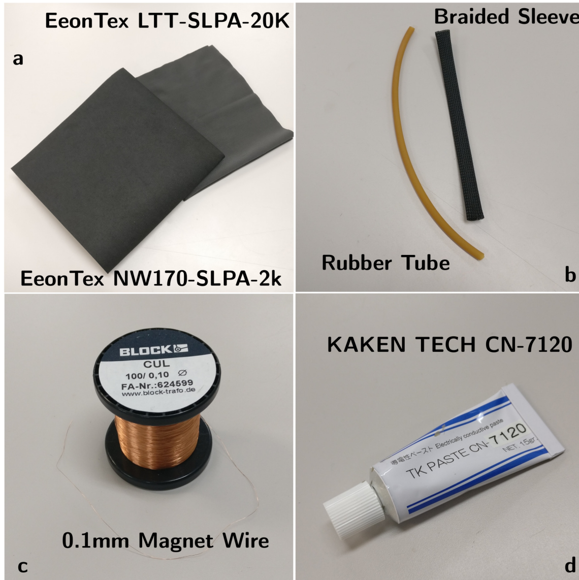
Figure 3.3: The images above display the materials, which were finally used for the artificial muscle spindle. Image a shows the conductive fabrics, and b the inner tube made of rubber as well as the outer braided sleeve. In image c magnet wire is shown and d shows the conductive adhesive that was used.
