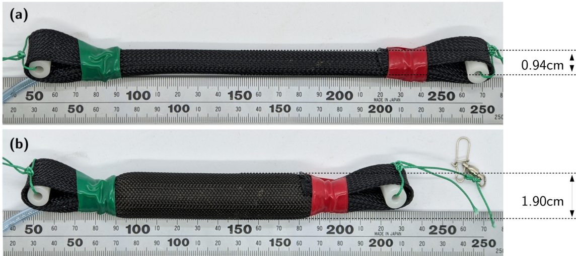
Figure 4.2: This image shows a pneumatic artificial muscle (PAM) in its deflated (a) and inflated (b) states. This actuator, with a diameter of 10\text{mm} , shortens by 40\text{mm} when pressurized with 0.7\text{MPa} .
