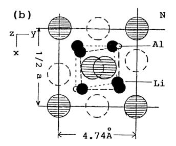
Fig. 29. Comparison of the structure: (a) projection of  $\alpha$ -Li<sub>3</sub>BN<sub>2</sub> structure along Z axis, (b) projection of antifluorite structure unit of Li<sub>3</sub>AlN<sub>2</sub>.
