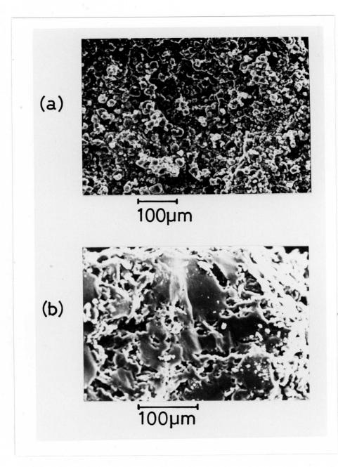
Fig. 5. SEM fracture photographs of sintered  $\text{Li}_3\text{AlN}_2$ bodies obtained at 1025 K (a) and at 1175 K (b).
