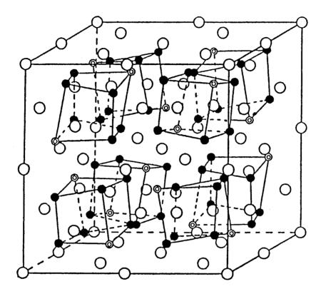
Fig. 4. Crystal structure of  $\text{Li}_3\text{AlN}_2$ . O Al, O Li,  $\bigcirc$  N.
