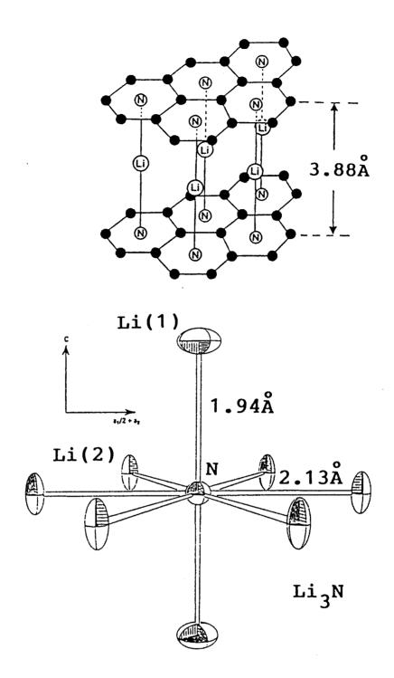
Fig. 30. Crystal structure of Li<sub>3</sub>N.
