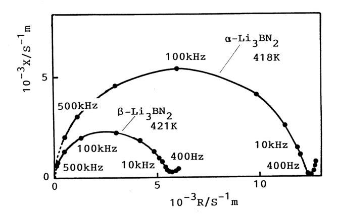
Fig. 34. Complex impedance plots for the polycrystalline  $\alpha$ -Li<sub>3</sub>BN<sub>2</sub> at 418 K and  $\beta$ -Li<sub>3</sub>BN<sub>2</sub> at 421 K.
