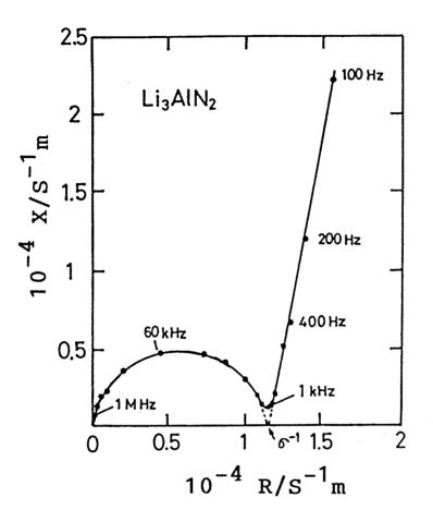
Fig. 6. Complex impedance plot at 343 K for the sintered  $\text{Li}_3\text{AlN}_2$ .
