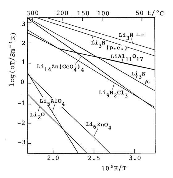
Fig. 2. Compilation of representative solid lithium ion conductors. The product of the conductvity  $\sigma$  and the absolute temperature T is plotted against the inverse absolute temperature.
