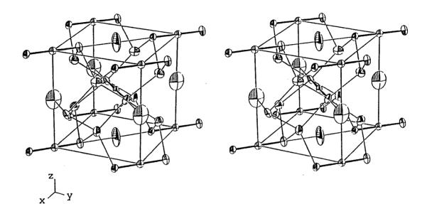
Fig. 27. Stereoscopic view of  $\alpha$ -Li<sub>3</sub>BN<sub>2</sub> structure.
