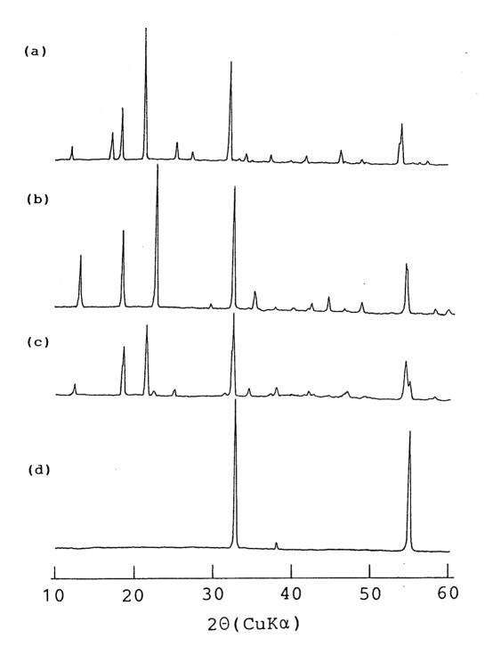
Fig. 12. X-Ray powder diffraction patterns of (a)  $\text{Li}_8 \text{SiN}_4$ , (b)  $\text{Li}_{21} \text{Si}_3 \text{N}_{11}$ , (c)  $\text{Li}_{18} \text{Si}_3 \text{N}_{10}$ , (d)  $\text{Li}_5 \text{SiN}_3$ .
