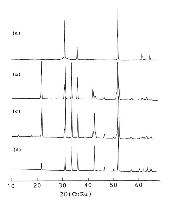
Fig. 18. X-Ray powder diffraction patterns of (a) LiMgN, (b) Li-Mg-N of No. 7 and (c) that of No. 8 in Table 15 and (d) Mg<sub>3</sub>N<sub>2</sub>.
