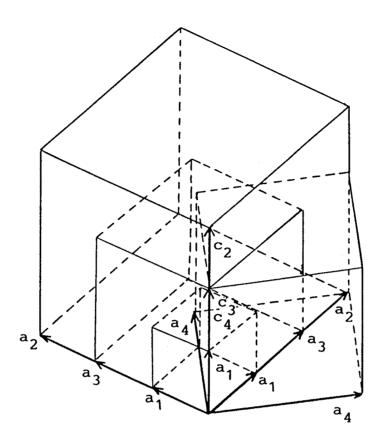
Fig. 13 Relationship of the unit cells;
