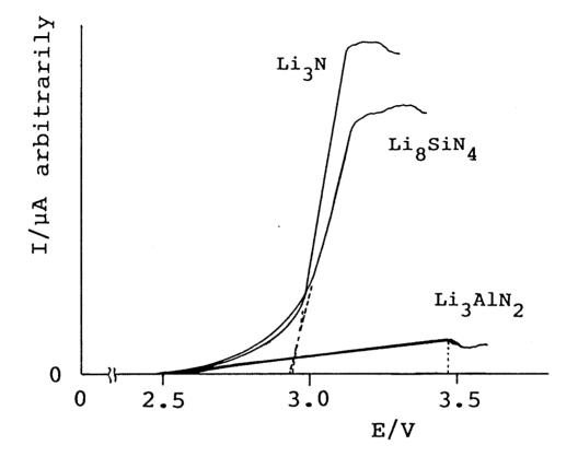
Fig. 39. Current against applied voltage on (-)Li solid elecrolyte C(+) cell at 375-385 K.
