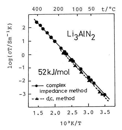
Fig. 7. Semilogarithmic plot of the product of conductivity  $\sigma$  and absolute temperature T against the inverse absolute temperature. The solid and the dotted lines represent the results obtained by complex impedance and by d.c. methods, respectively.
