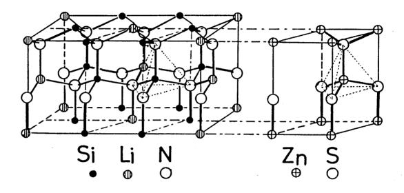
Fig. 10. Crystal structure of  $\text{LiSi}_2N_3$  compared with that of wurtzite.
