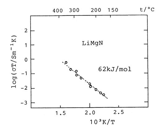
Fig. 19. Temperature dependence of the conductivity for LiMgN.
