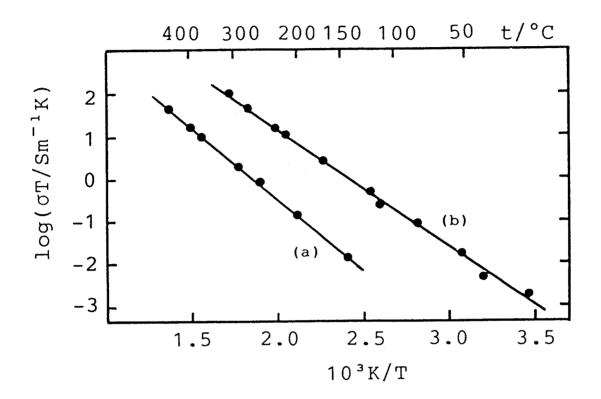
Fig. 15. Semilogarithmic plot of the conductivity  $\sigma$  times the absolute temperature T against the inverse absulte temperature: (a) LiSi<sub>2</sub>N<sub>3</sub> and (b) Li<sub>2</sub>SiN<sub>2</sub>.
