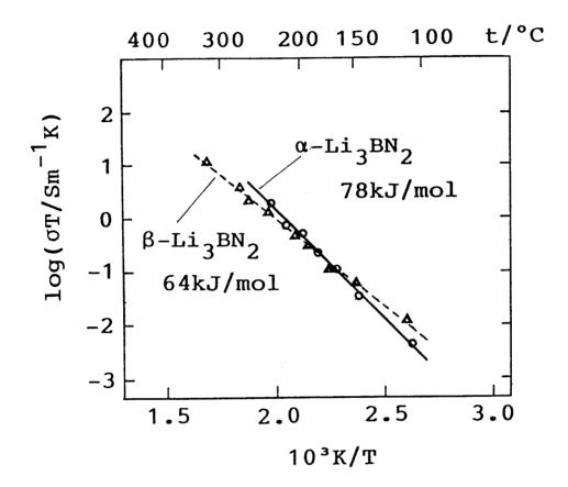
Fig. 35. Semilogarithmic plot of the conductivity σ times the absolute temperature T against the inverse absolute temperature.
