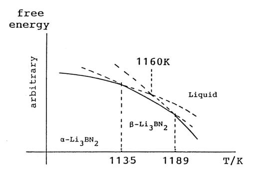
Fig. 23. Schematic free energy curves of  ${\rm Li}_3{}^{\rm BN}{}_2$  against temperature.
