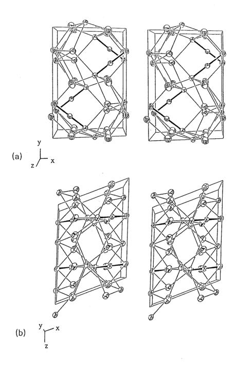
Fig. 24. Stereoscopic views down [001] (a) and [010] (b) of the  $\beta$ -Li<sub>3</sub>BN<sub>2</sub> structure. The 70% probability thermal ellipsoids for all atoms are shown. No atoms are labeled, but straight N-B-N bonds are obvious because of their thicker bonds which denote covalent B-N bonds. Larger ellipsoids are Li(1) and Li(2). Table 25. Interatomic distances (Å) and angles (•) with estimated standard errors given in parentheses.
