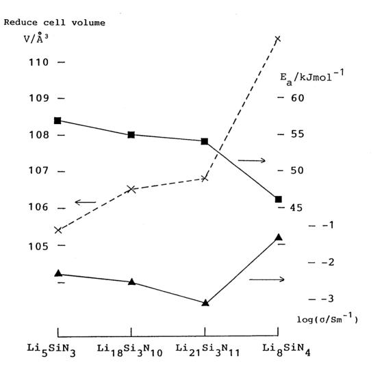
Fig. 14. Compositional dependence of reduced cell volume, activation energy of ionic conduction and ionic conductivity at 400 K among the lithium silicon nitrides.
