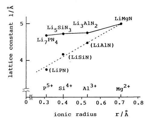
Fig. 36. Lattice constants of elemental cell versus ionic radii. The value of imaginary compounds (LiAlN), (LiSiN) and (LiPN) are obtained from Fig. 35.
