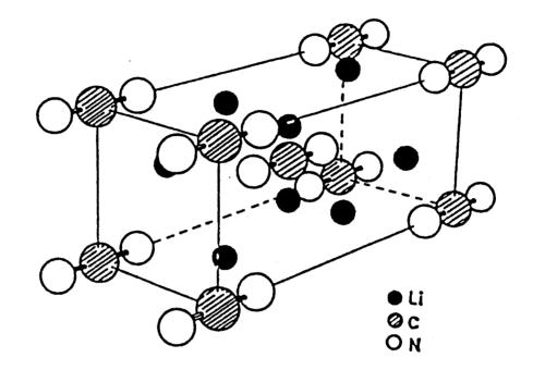
Fig. 33. Crystal structure of Li<sub>2</sub>CN<sub>2</sub>.
