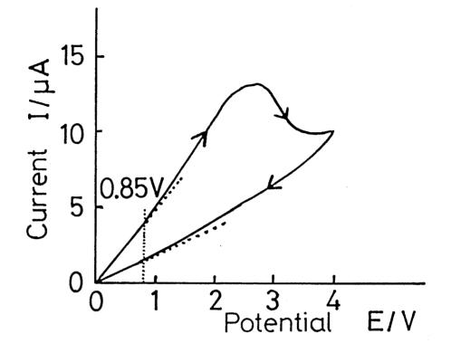
Fig. 8. Current against applied voltage on Li/Li<sub>3</sub>AlN<sub>2</sub>/Li cell at 377 K.
