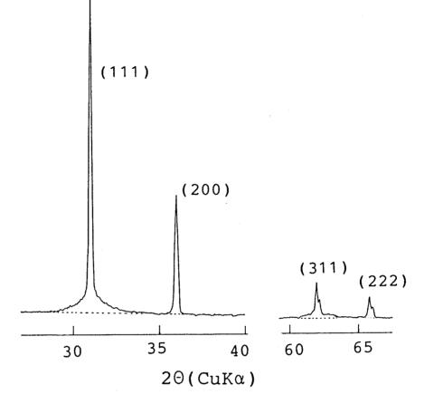
Fig. 17. X-ray powder diffracion pattern of LiMgN.
