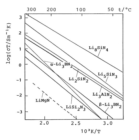
Fig. 38. Ionic conductivity in a series of double metal nitrides containing lithium.
