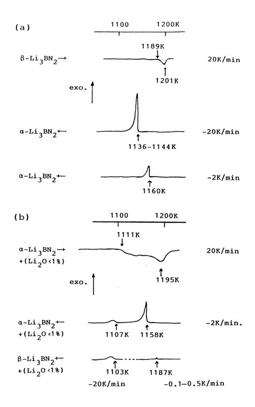
Fig. 22. Differential thermal analyses of (a)  $\beta$ -Li<sub>3</sub>BN<sub>2</sub> single crystals (0.3-1.0 mm) and (b)  $\alpha$ -Li<sub>3</sub>BN<sub>2</sub> polycrystalline containing Li<sub>2</sub>O<1 wt%.
