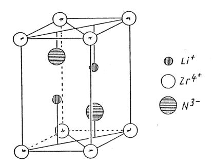
Fig. 11. Crystal structure of Li<sub>2</sub><sup>ZrN</sup><sub>2</sub>.
