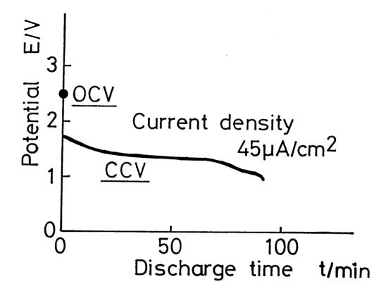
Fig. 9. Discharging of Li  $|\text{Li}_3\text{AlN}_2|$  TiS<sub>2</sub> at 377 K.
