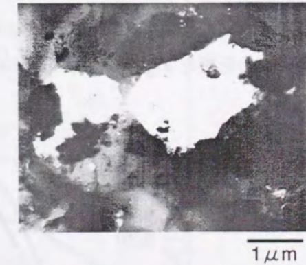
Fig. 2.2 TEM micrograph of Al-17Si-4.5Cu-0.5Mg P/M alloy.
