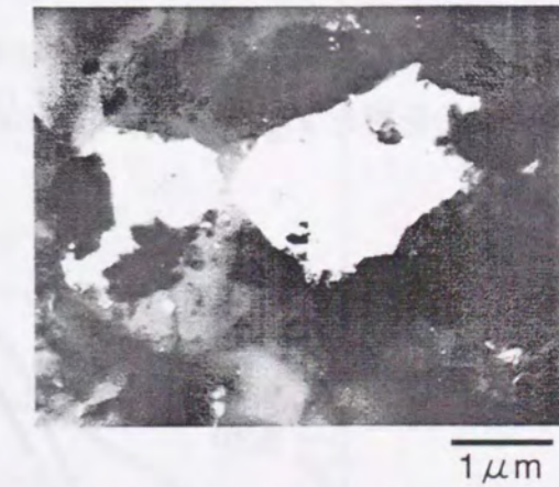
Fig. 2.2 TEM micrograph of Al-17Si-4.5Cu-0.5Mg P/M alloy.
