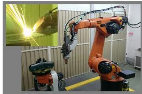
Experimental apparatus for laser cladding
