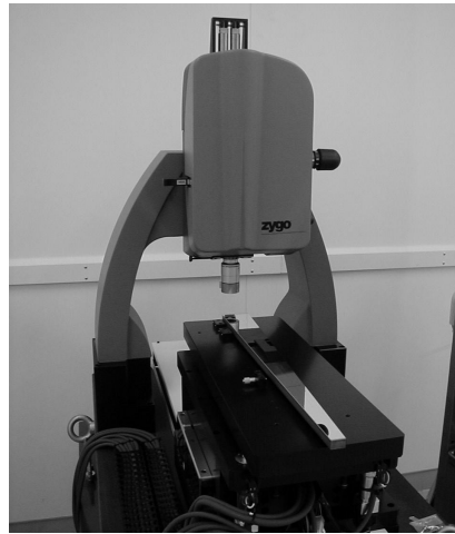
Fig. 1. Photograph of the MSI for the half-meter-long mirror. The 5-axis stage is placed under a microscopic interferometer head (Zygo Corp., NewView 5000). A test trapezoidal mirror of length 540mm is set on the stage.
