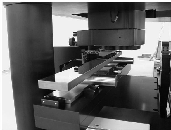
Fig. 4. Photograph of the right-side view of the image in Fig. 3. A test mirror of length 540 mm and a reference mirror of length 100mm are placed on each stage under the Fizeau interferometer.
