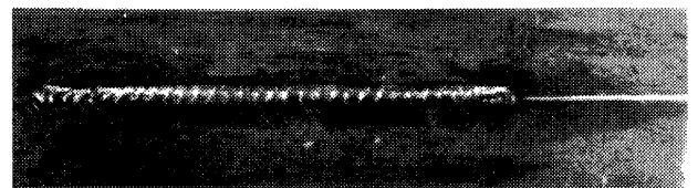
Fig.6 A welding result of pulsed MIG/MAG welding with Pulsed wire feeding
