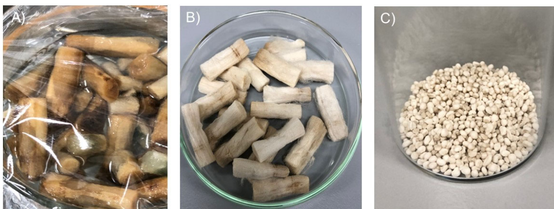
Figure 2-2. Pictures of the steps taken from used CFs (A) to MCBs (C) through recycled CA fibers (B)
