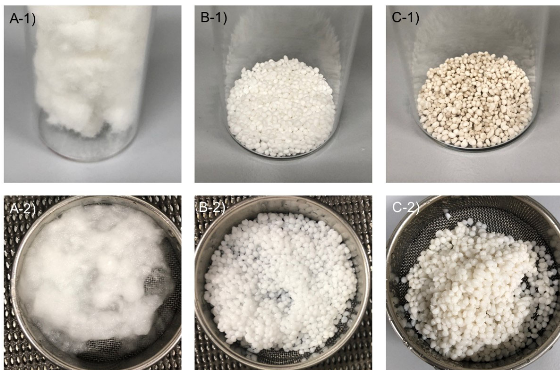
Figure 2-8. Absorption images of fluff pulp (A), MCB-3 (B), and MCB-4 (C)
