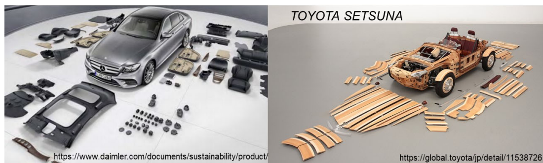
Figure 2. Automobile components made of NFRCs
