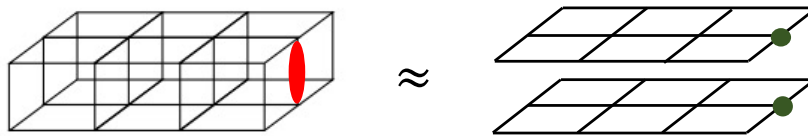
FIGURE 5.1: Schematic representation of the correspondence between a two-layer PDM and two 2D MDMs.
