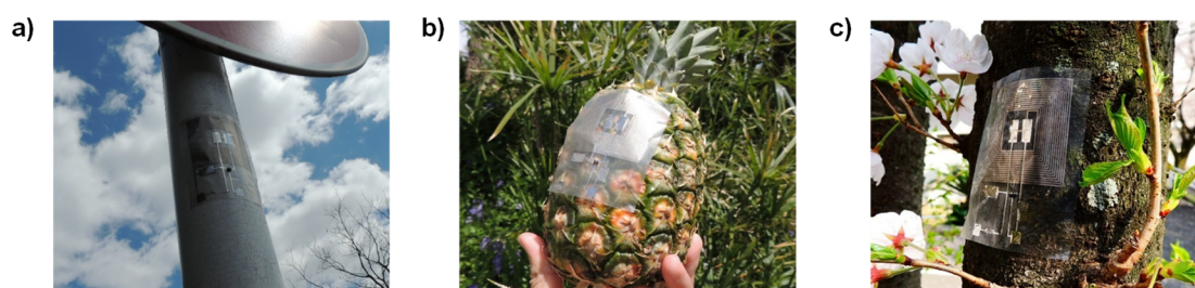
Fig. 2-8 Examples of the potential uses of nanopaper sensor devices such as a) a hyperdense meteorological observation network, b) real-time monitoring of the storage conditions of packages, such as agricultural products, and c) efficiency improvement of forestry by monitoring the growth of individual trees, environmental forecasting, and measurement.
