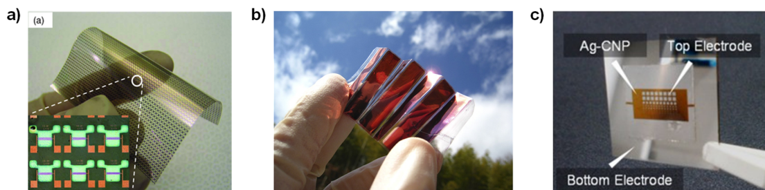
Fig. 10. a) Nanopaper-based transistors, b) solar cells, and c) memories. Reprinted and modified from references 73, 74, 75.
