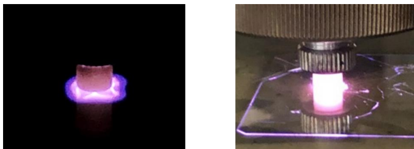
Figure 3.5 Photograph of plasma generated on ultra-thin quartz crystal wafer using Ar as the carrier gas.
