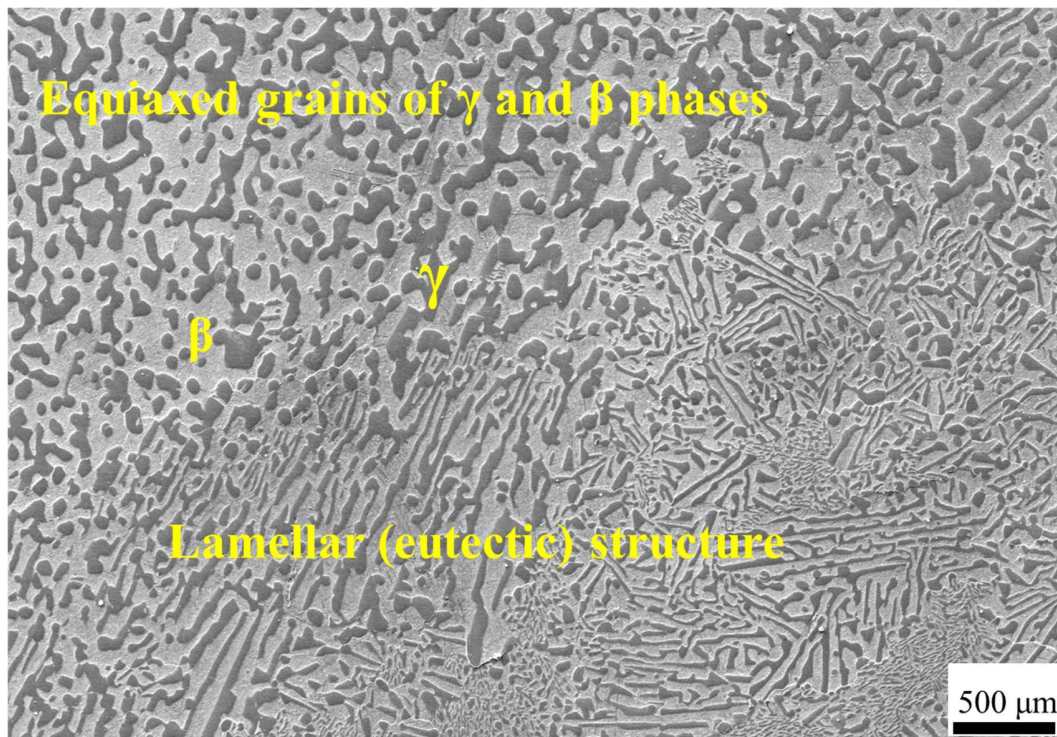
Figure 1.8 A typical microstructure of the eutectic In52Sn48 alloy.
