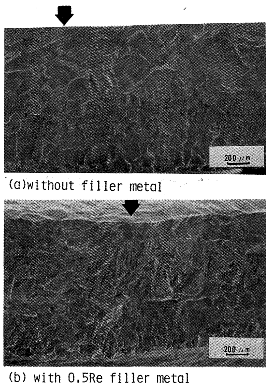
Fig. 10 SEM fractograph of AM-TZM welds without or with Re filler after Trans-bend test.
