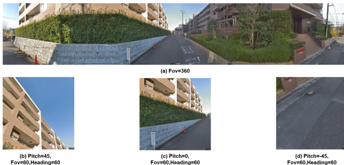
Figure 4.10 GSV images for a sampling point with different vertical viewing angles (i.e., pitches): (a) panoramic street view image, fov = 360; GSV images with (b) pitch = 45, fov = 60, heading = 60; (c) pitch = 0, fov = 60, heading = 60; (d) pitch = -45, fov = 60, heading = 60.
