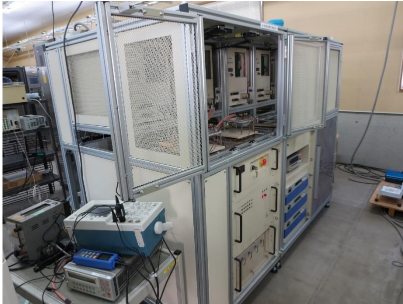
Fig. 3.9 Power cycling tester.
