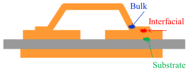
Fig. 4.19 Destruction modes by pull test.
