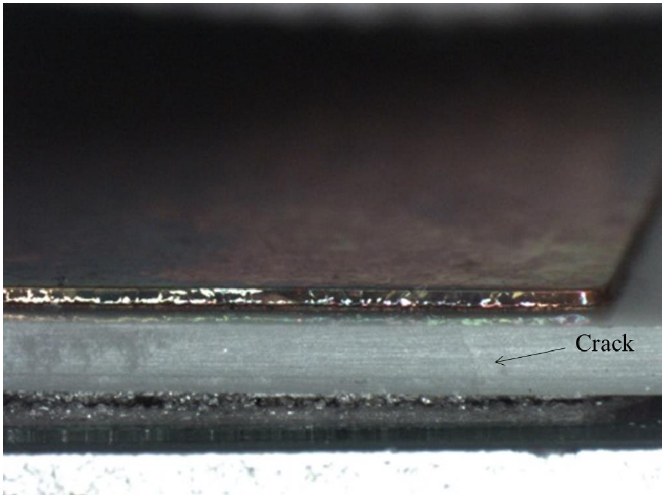
Fig. 4. 29 Vertical crack in AlN after 300 cycles.
