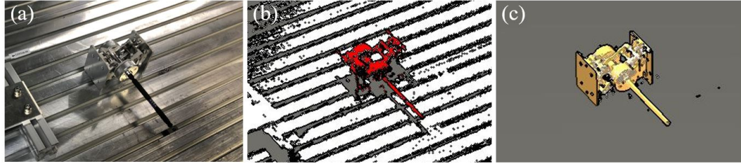
Figure 4.20: (a) The tool on a table. (b) White: Background point cloud; Red: Tool point cloud. (c) The tool pose found by matching the tool's mesh model to the red point cloud.
