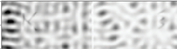
FIGURE 5. Energy distribution for the burst wave at 20 kHz
