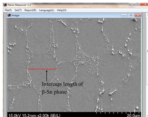
Fig. 4-1 Typical example of the mean intercept length measurement.
