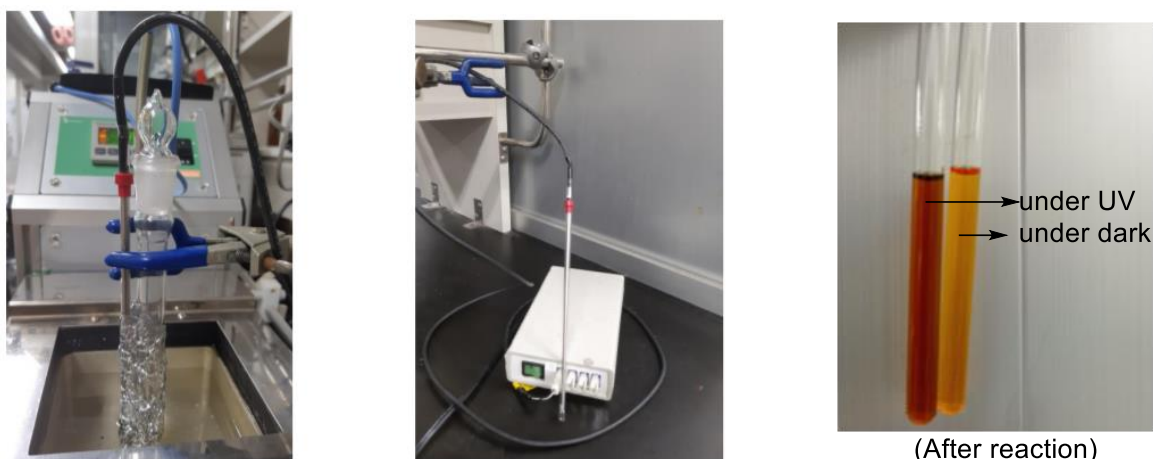
Figure 23. Reaction setting with LED (left), apparatus (PER-AMP) (middle), and the color change observed after reaction under dark and UV.
