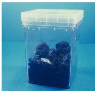
Figure 3-1. PLA film degradation test with the compost in a jar.
