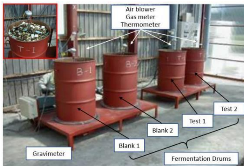
Figure 4-2. A photograph of the pilot-scale compost apparatus. (left) Two drums are the blank zone without PLA samples and (right) two drums are the test zone with PLA samples. All drums were equipped with an air blower, gas concentration meter, and thermometer. Drums were placed on a gravimeter.
