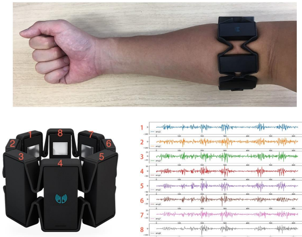
Figure 2.2: Myo Armband setup (top), correspondence of Myo Armband EMG sensors to their signals (bottom).
