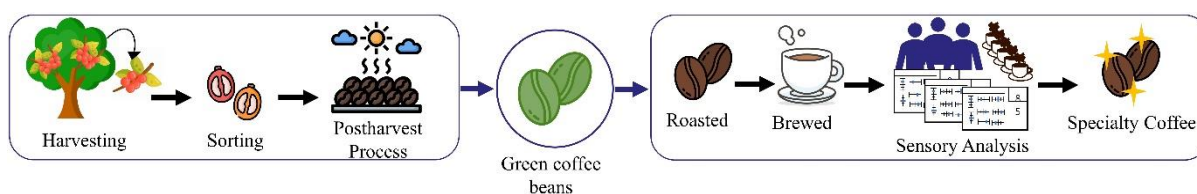
Figure 1.2-1 The production process of Arabica coffee from cherry to cup. In specialty coffee Arabica production, the sensory analysis is conducted to determine the coffee beans grade.
