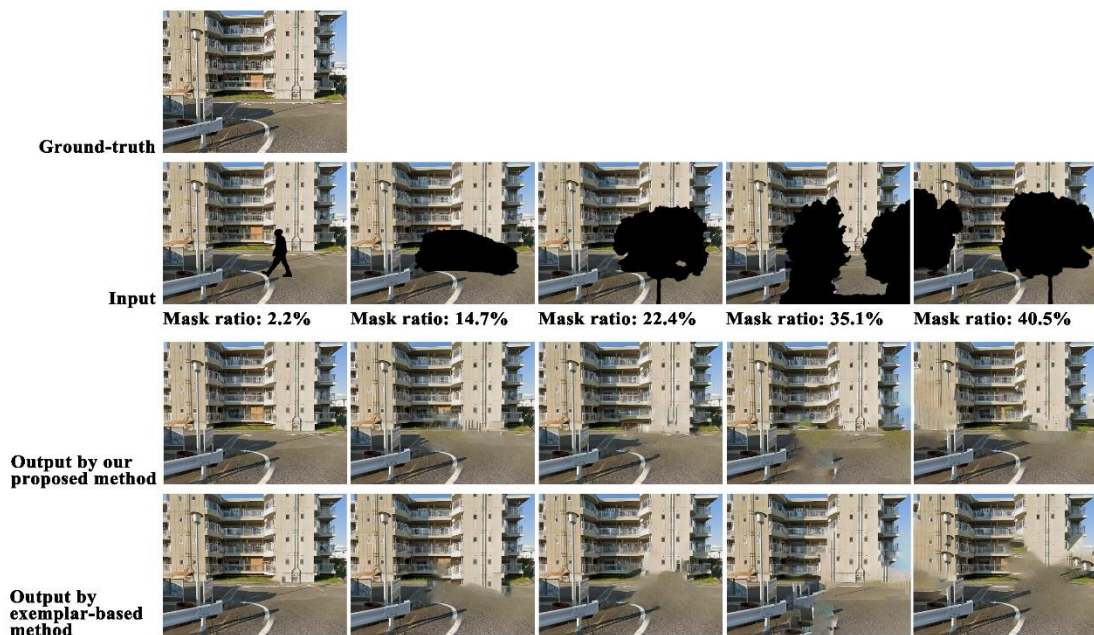
Figure 3.8. Validation examples of automatic object removal and facade completion.
