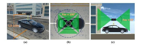
Figure 4.6. Virtual car setup used for data acquisition. One virtual multi-cameras with four perspectives are used. The horizontal and vertical view angles are 100 degrees and 79 degrees.
