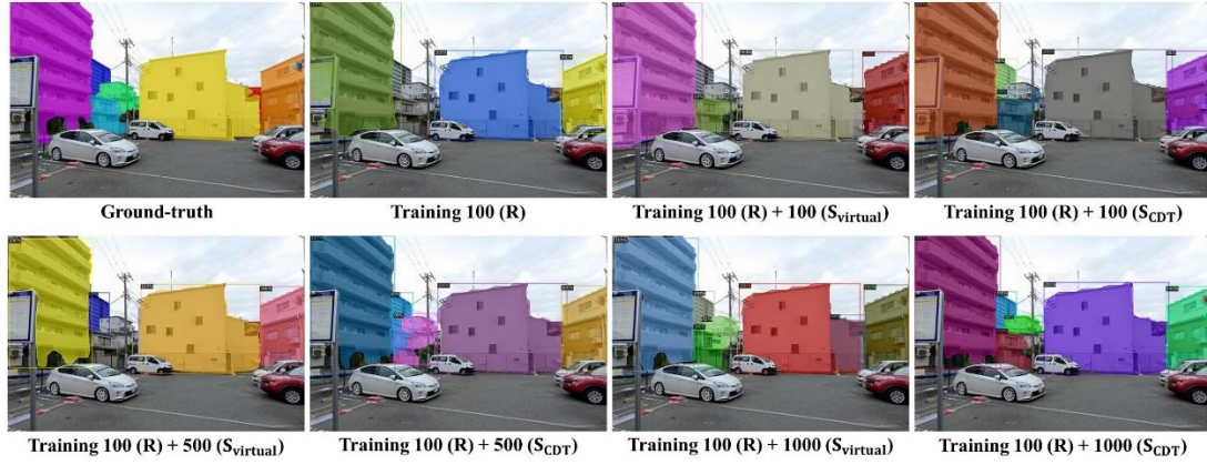
Figure 4.11. Qualitative results for training real datasets only and for extending them with the two types of synthetic datasets (CDT and virtual).
