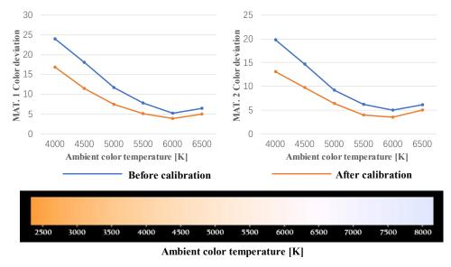
Figure 5.10. Color deviation of two materials in several color temperatures before and after photo color calibration.
