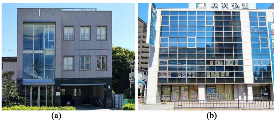
Figure 5.18. Some observations from street view images illustrate the limitations of facade segmentation. (a) The window glass reflects trees, and (b) the window glass reflects buildings will reduce the segmentation accuracy of walls and windows.
