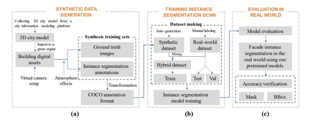
Figure 4.2. Workflow for the study: (a) the synthetic data generation process, (b) training DCNN-based instance segmentation, and (c) evaluation using real-world imagery.
