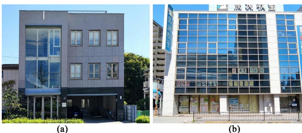
Figure 5.18. Some observations from street view images illustrate the limitations of facade segmentation. (a) The window glass reflects trees, and (b) the window glass reflects buildings will reduce the segmentation accuracy of walls and windows.
