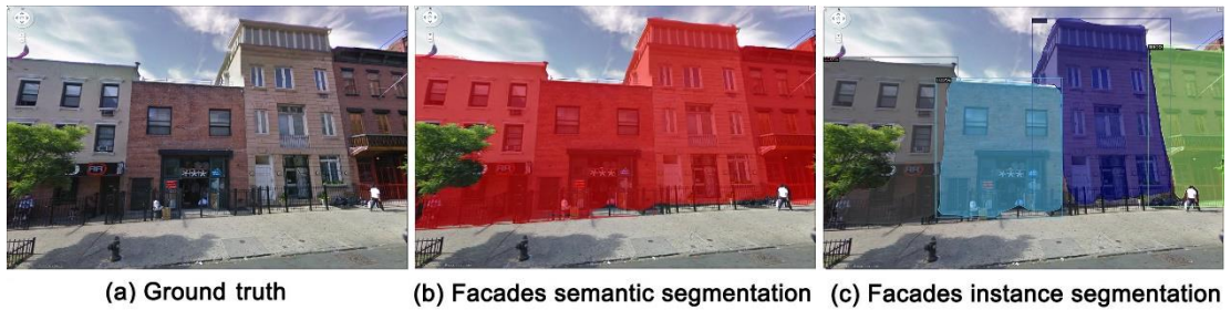
Figure 5.6. Compared to facade extraction methods that use semantic segmentation, instance segmentation can extract building facade information one by one when multiple buildings are connected in a single image. (a) Ground truth, (b) facade semantics segmentation, (c) facade instance segmentation.
