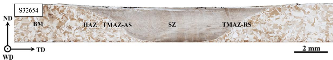
Figure 1.15 Etched weld section of FSW joints [117]
