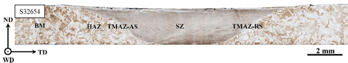
Figure 1.15 Etched weld section of FSW joints [117]
