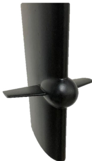
Fig 2-6 Scaled RBFS model
