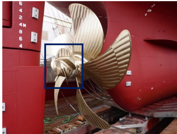
Fig 1-4 Propeller boss cap fins (Source: www.greenaward.org )
