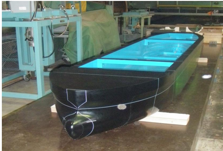
Fig 3-8 KVLCC2 tanker model (Mwangi, 2021)
