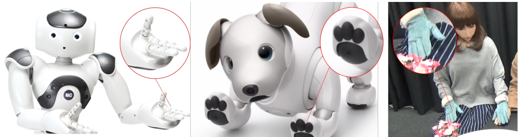
Figure 5.1: (Left) NAO with a three finger hand; (Middle) AIBO with a paw; (Right) ERICA the android with human-like hands; (NAO's Image modified from https://aibo.sony.jp/ ) (AIBO's Image from https://bit.ly/3MHg71b )
