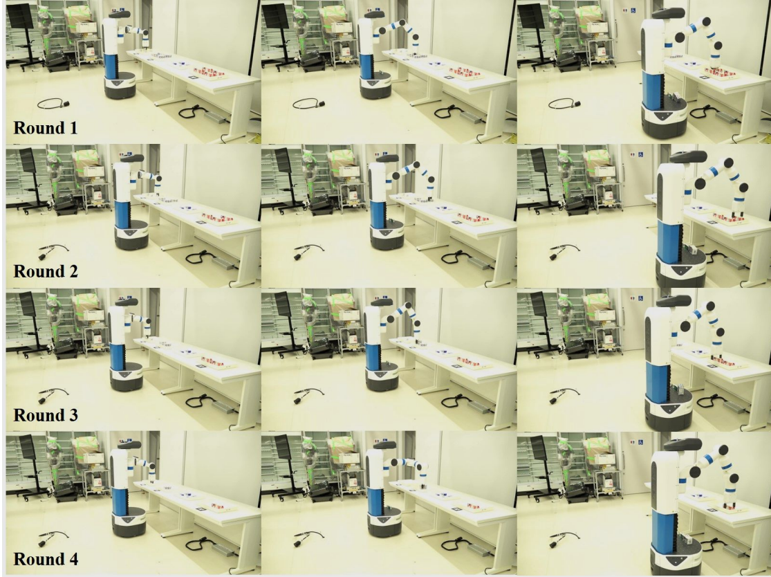
Figure 3.26: The base positions update based on the target objects to be picked, the update is performed after every round of pick-and-place tasks.
