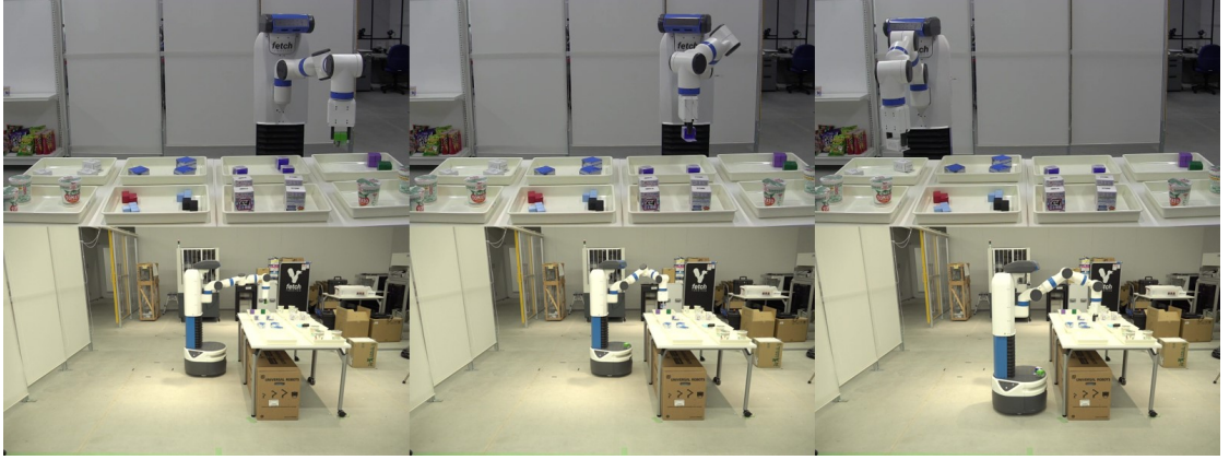
Figure 3.19: (Left and Middle) Move to P_{B1} \cap P_{B2} to pick up parts from tray_1 and tray_2 . (Right) Move to P_{B4} to pick up a part from tray_4 .
