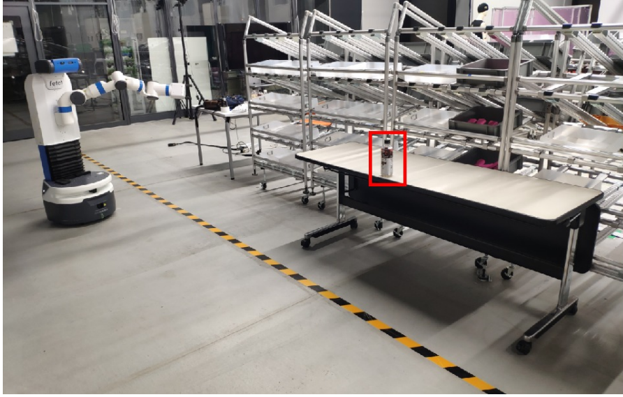
Figure 4.11: The overview of the experiment. The task is to use push-grasp to pick up a bottle from a table.
