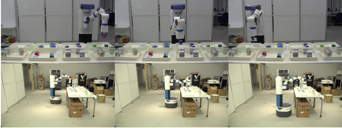
Figure 3.18: (Left) Move to P_{B1} to pick up a part from tray_1 . (Middle) Move to P_{B2} to pick up a part from tray_2 . (Right) Move to P_{B4} to pick up a part from tray_4 .
