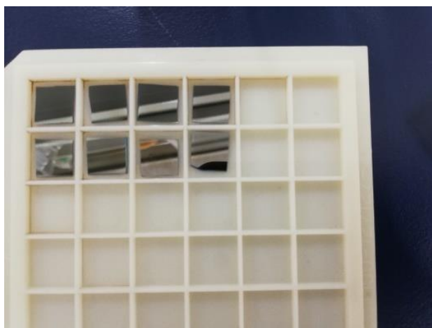
Figure 2.1 The photo of cleaned \text{SiO}_2/\text{Si} substrate ( \sim 10 mm square) uniformly dropped with 20 \mu\text{l} -NDs.
