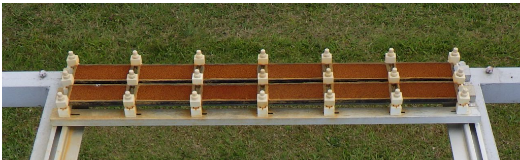
Figure 2-3. The appearance of the atmospheric exposure test.
