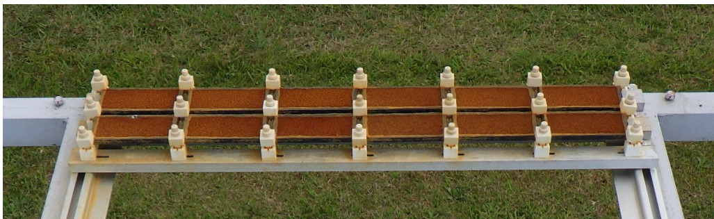
Figure 2-3. The appearance of the atmospheric exposure test.
