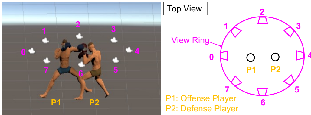
Figure 5.11: The candidate viewpoints setting in this implementation: 8 candidate viewpoints are set on the view ring evenly, and 45 degrees between the two candidate viewpoints.
