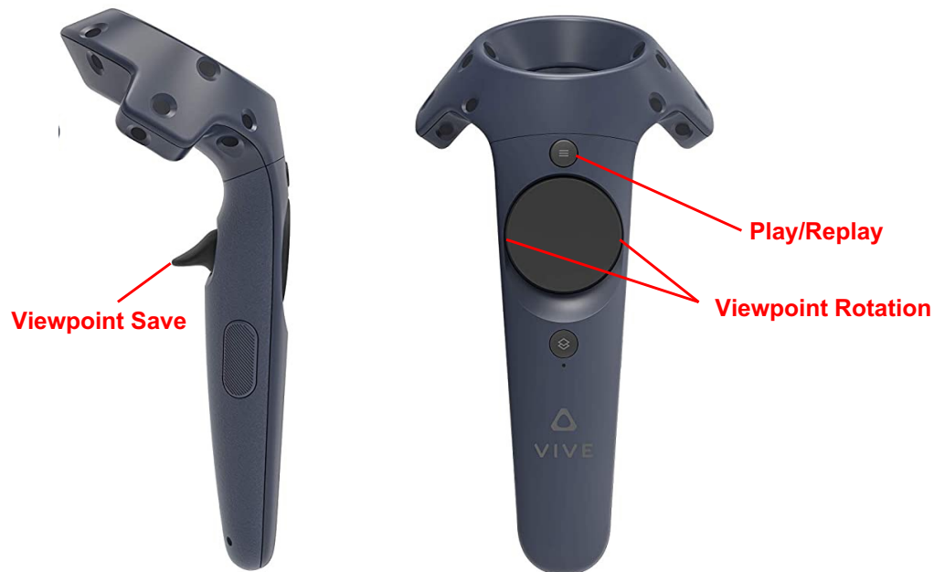
Figure 5.9: Using one HTC Vive controller for viewpoint selection in experiment: Menu button is set for playing and replaying the videos; Touchpad is set for rotating the viewpoint on the view ring; Trigger is set for saving the selected preferred viewpoint.
