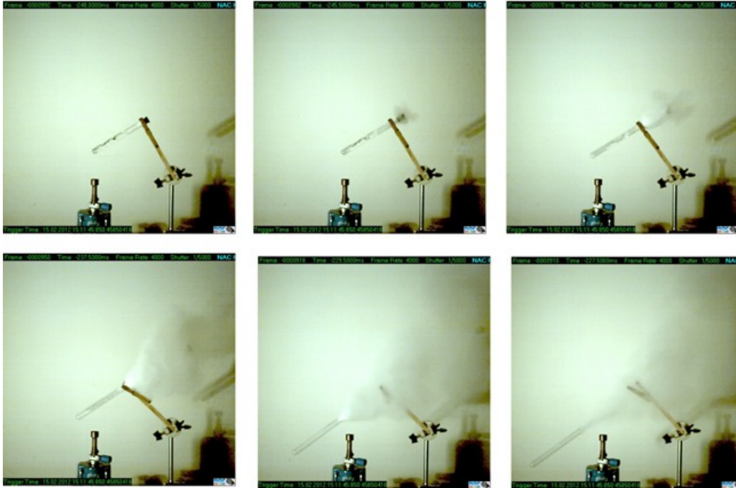
Figure 2.1: Ejection of a rubber stopper from a test tube due to vapour pressure: Sequence of snapshots recorded with 4000 Hz/shutter 1/5000 s at the following times: t = 0, + 2.5 \text{ ms}, + 5.5 \text{ ms}, + 10.5 \text{ ms}, + 18.5 \text{ ms}, + 20.5 \text{ ms} [Vollmer and Möllmann (2012b)].
