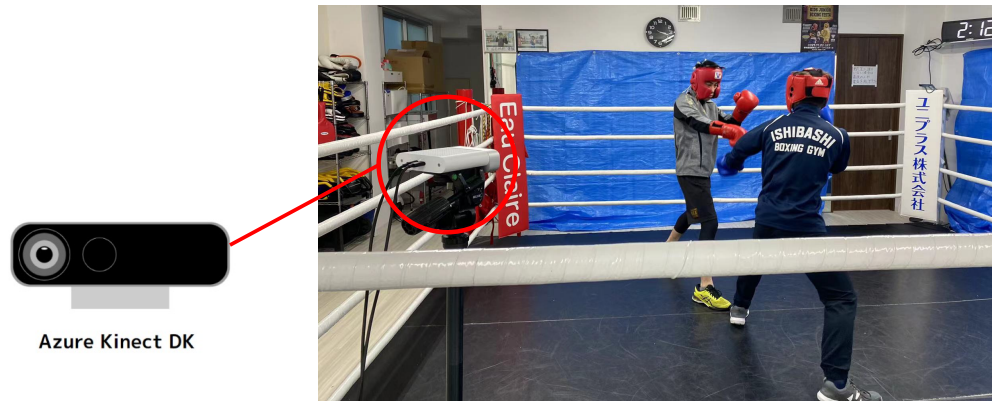
Figure 5.8: The Azure Kinect depth camera setting for boxing punch scene recording: one Azure Kinect depth camera is set in the corner of the boxing ring.
