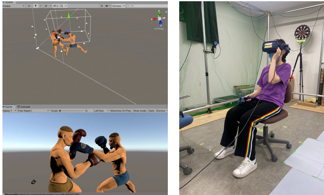
Figure 5.10: A labeling experiment for collecting the user preferred viewpoint in different preference condition: left top is scene view of the experiment program, left bottom is the view in VR device which the user can see, right shows that a participant takes part in the experiment who is sitting on a chair and using a controller to select preferred viewpoint.
