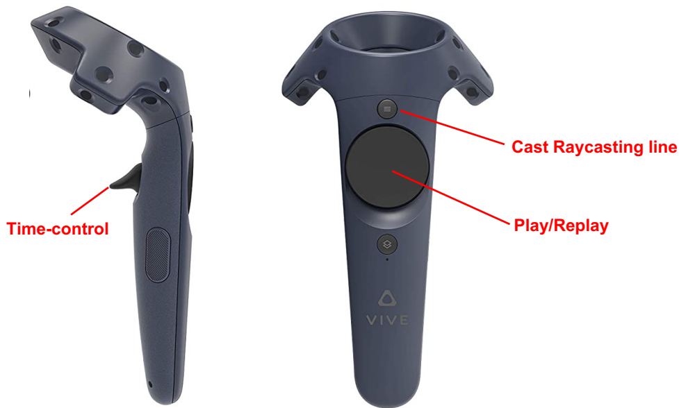
Figure 3.5: The HTC Vive controller setting for interaction: the Touchpad is set for pltheay or replay the videos; Menu button is set for casting a Raycasting line; the Trigger is set for the time-control.
