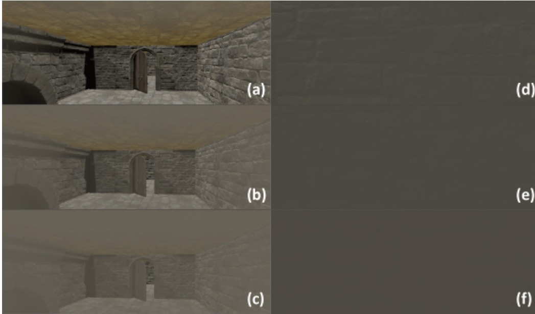
Figure 3.3: The effect of the vision modulator during continuous locomotion with different parameters. The left column shows views when facing distant objects, with parameters of (a) CR=10 , (b) CR=20 , (c) CR=30 . The right column shows the effect when a wall is directly in front of the camera, with parameters of (d) CR=10 , (e) CR=20 , (f) CR=30 .
