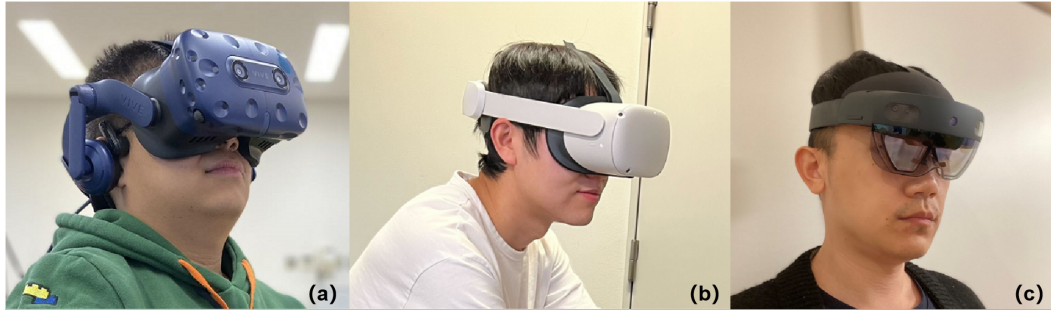
Figure 1.1: Images of the immersive HMDs and OST-HMD applied in this work. (a) The HTC Vive Pro Eye and (b) Oculus Quest 2, which provide the user with a fully-immersive VR experience and hence prevent the user from directly viewing the real world. (c) A user wearing the Microsoft HoloLens 2, which renders digital content directly in the user’s field of view overlaid onto the real world.
