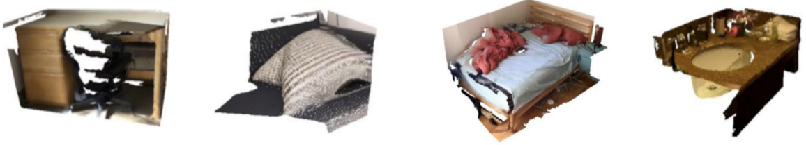
Fig. 4.5 Some example point clouds from the OBJ_BG dataset of ScanObjectNN. The data therein is challenging for containing noise, holes, deformations, and incompletely removed backgrounds.
