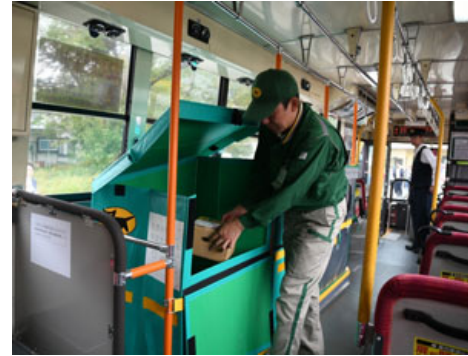
(B) A delivery driver loading cargo into a remodeled cargo space inside the bus. Source: Yamato Transport (Yamato-Holdings, 2018)
