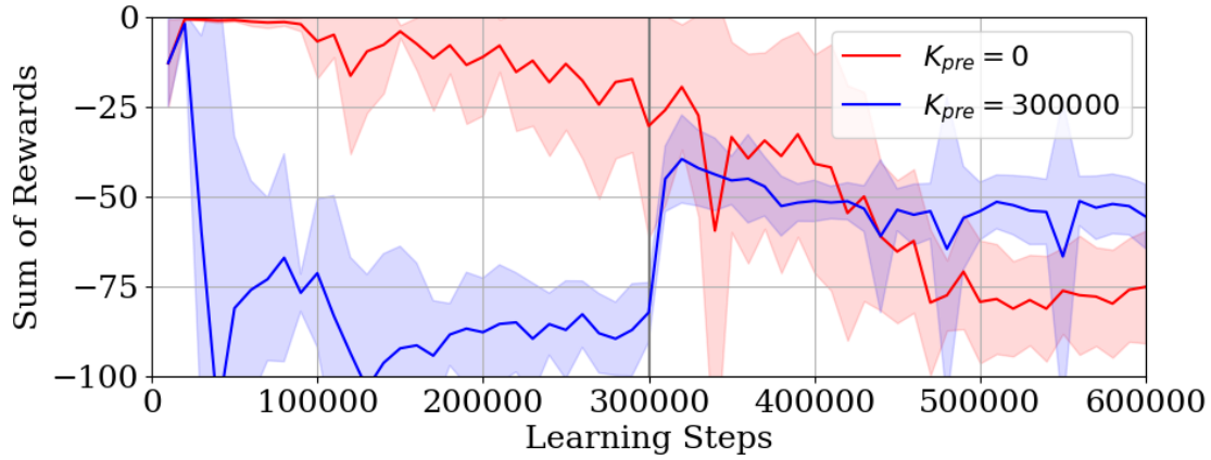
Fig. 6.5: Reward learning curves for the formula \Phi_1 . The red and blue curves show the results of K_{pre} = 0 ( Case 1 ) and K_{pre} = 300000 ( Case 2 ), respectively. The solid curves and the shades represent the average results and the standard deviations over 10 trials with different random seeds, respectively. The gray line shows 300000 steps.
