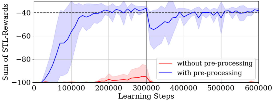
Fig. 6.12: STL-reward learning curves for the case without pre-processing (red) and the case with pre-processing (blue). We consider the formula \Phi_1 . The solid curves and the shades represent the average results and the standard deviations over 10 trials with different random seeds, respectively. The dashed line shows the threshold l_{STL} = -40 . The gray line shows 300000 steps.
