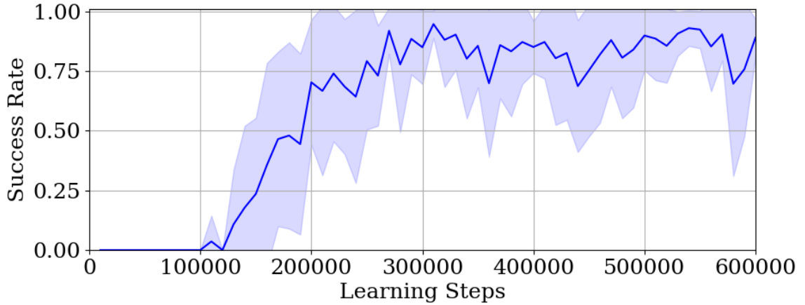
(b) Success rate for the environment with random delays. The solid curve and the shade represent the average results and the standard deviations over 10 trials with different random seeds, respectively.
