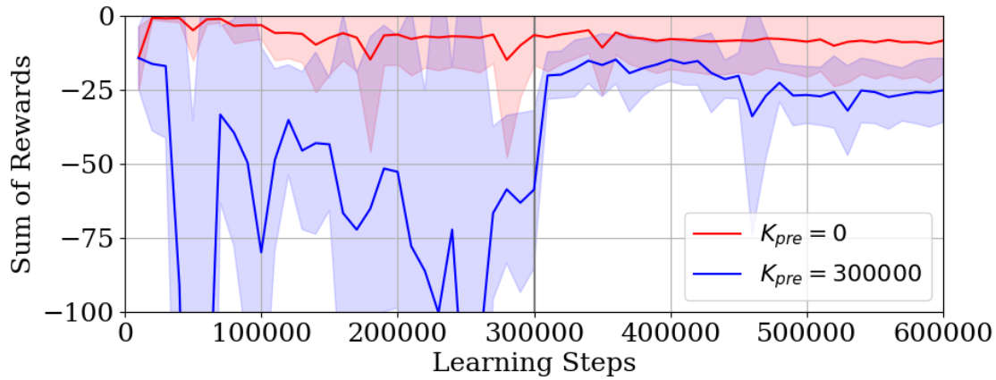
Fig. 6.9: Reward learning curves for the formula \Phi_2 . The red and blue curves show the results of K_{pre} = 0 ( Case 1 ) and K_{pre} = 300000 ( Case 2 ), respectively. The solid curves and the shades represent the average results and the standard deviations over 10 trials with different random seeds, respectively. The gray line shows 300000 steps.
