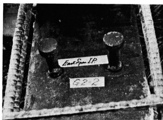
(a) 余盛止端部の疲労亀裂 (G 2-2)
