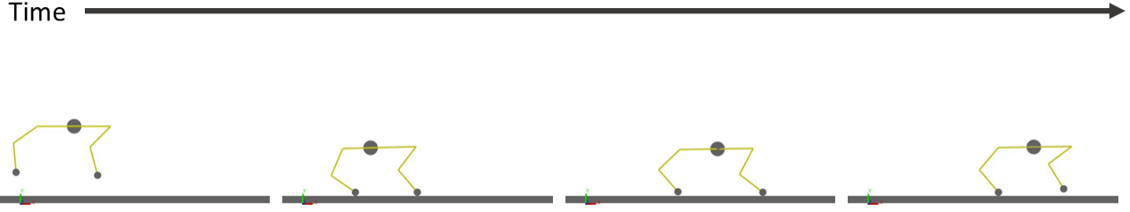
Figure 3: Snapshot of the robot running every 500.0 [ms] with k^{ab} = 1.0 \times 10^2 [N/m].
